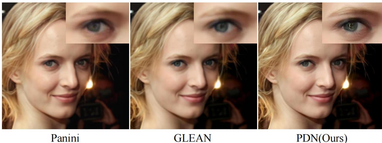
Figure 7: Results on unseen downsamplings. PDN yields clearer results when facing unseen downsamplings. Here the networks are all trained on 8\times bicubic(alias) and tested on 8\times bicubic(antialias).
